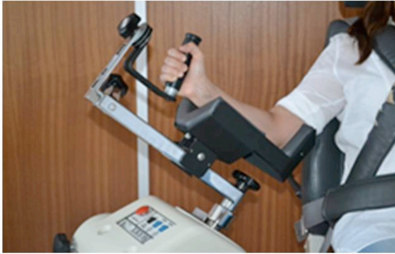
Figure 3. Measure of the strength internal and external shoulder rotators by means of an Isocinetic Dynamoter (Biodex Medical System).
