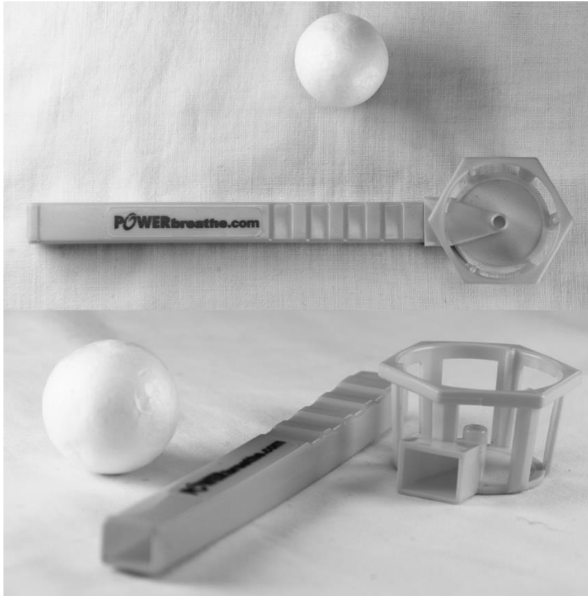
129 Figure 1. The flow-ball device used for the study ( www.powerbreathe.com ). A 140 mm 130 long tube with a rectangular cross section of 7 by 10 mm. A basket with a narrow, 131 upward facing opening of 3.9 mm diameter 12 mm is attached to the tube. The device 132 was supplied with a polystyrene ball of Ø 29 mm.
