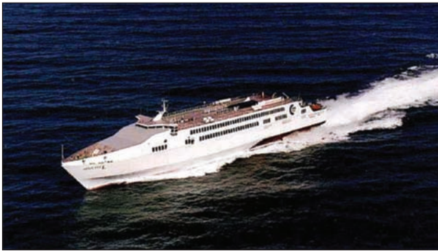
Figure 4. The high-speed ship. The vehicle is a 110-m-long, deep-V aluminium monohull ship, which carries 1,250 passengers at 40 kn. She uses waterjets and is operational in Europe and South America during the summer.
