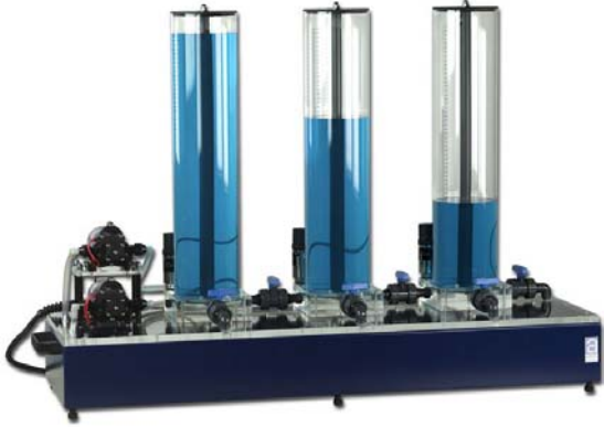
Fig. 1. The three-tank system by Amira.
