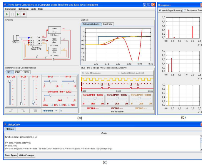
Fig. 6. Graphical user interface of the second example. Figures: (a) is the main view, (b) show histograms of input-output latencies or response time for three tasks, (c) is the dialogCode where the user can read and write the code of PID computation. Note the schedule data of the red task and its control performance
