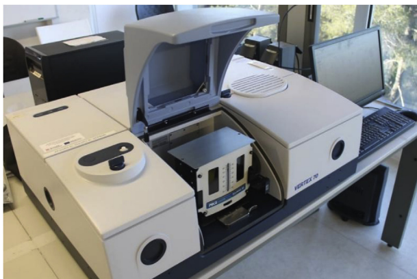
Fig. 2. Infrared reflection absorption spectroscopy (Vertex 70, Bruker).
