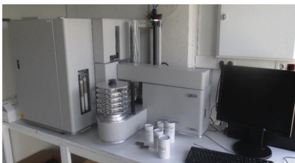
Fig. 1. Multi-phase carbon determination instrument (RC612, Leco).
