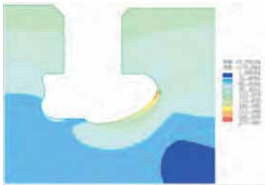
Figure 13 - HP Blade 1 groove, max Von Mises stress.
