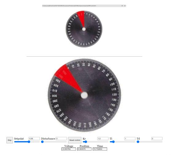
Fig. 6: Web app when the metadata is not available and the UI cannot be built automatically (top), and when it is (bottom). The *Stop* button is added by RIP automatically even if it is not defined in the server, and the server executes its action when the user presses this button in the app or when the client disconnects. This example uses EJS' default CSS configuration.
