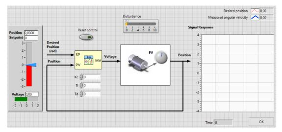
Fig. 4: Modified version of National Instruments' VI example for position control of a servo-motor. Required changes were: 1) replace the cluster control representing the PID with three float controls for each of the PID parameters, and 2) remove all repeated controls/indicators in any of their forms. The "Time" output was also added, not because it is required, but to explicitly provide this important information in the resulting web app.
