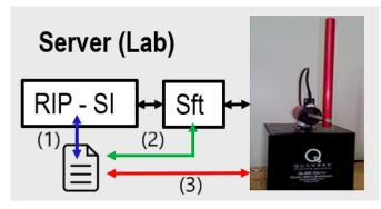
Fig. 1: Possible metadata sources: (1) custom-defined information in the configuration files of the RIP server implementation (RIP-SI), (2) lab software (Sft); either a simulation model or a control program, and (3) lab plant with IoT devices.
