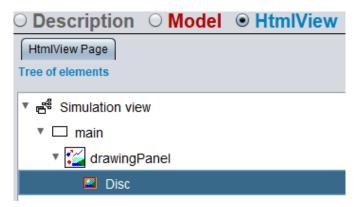
Fig. 5: Setup of the servo-motor web application in EJS. Defining the UI is reduced to inserting a main and a drawing panel (which correspond to  $\langle div \rangle$  tags in HTML), and an image of a disc to represent the motor in the virtual lab.
