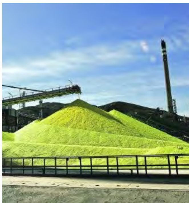
Figure 1. Excess Sulfur in an oil refinery
