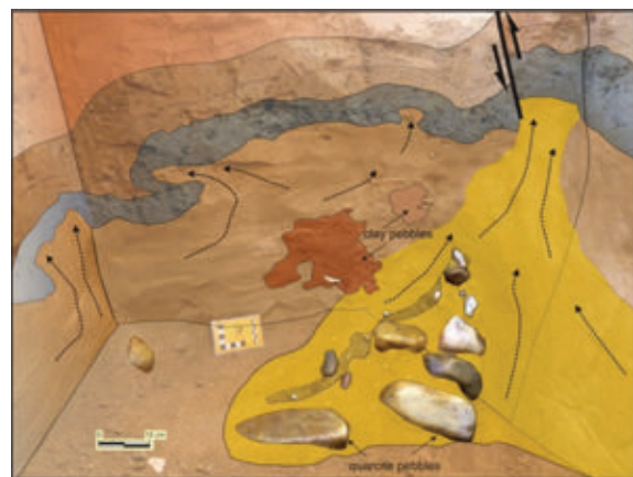
Figure 3: Photography and interpretational sketch of the liquefaction structures located under the cistern made of hydraulic mortar.
