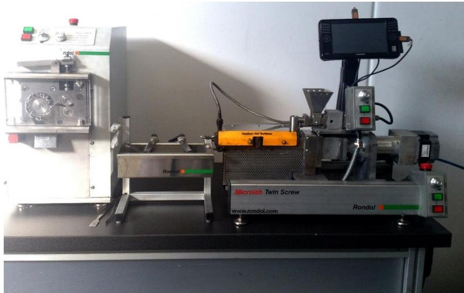
Figura 131. Micro-extrusora Rondol 10 mm.
