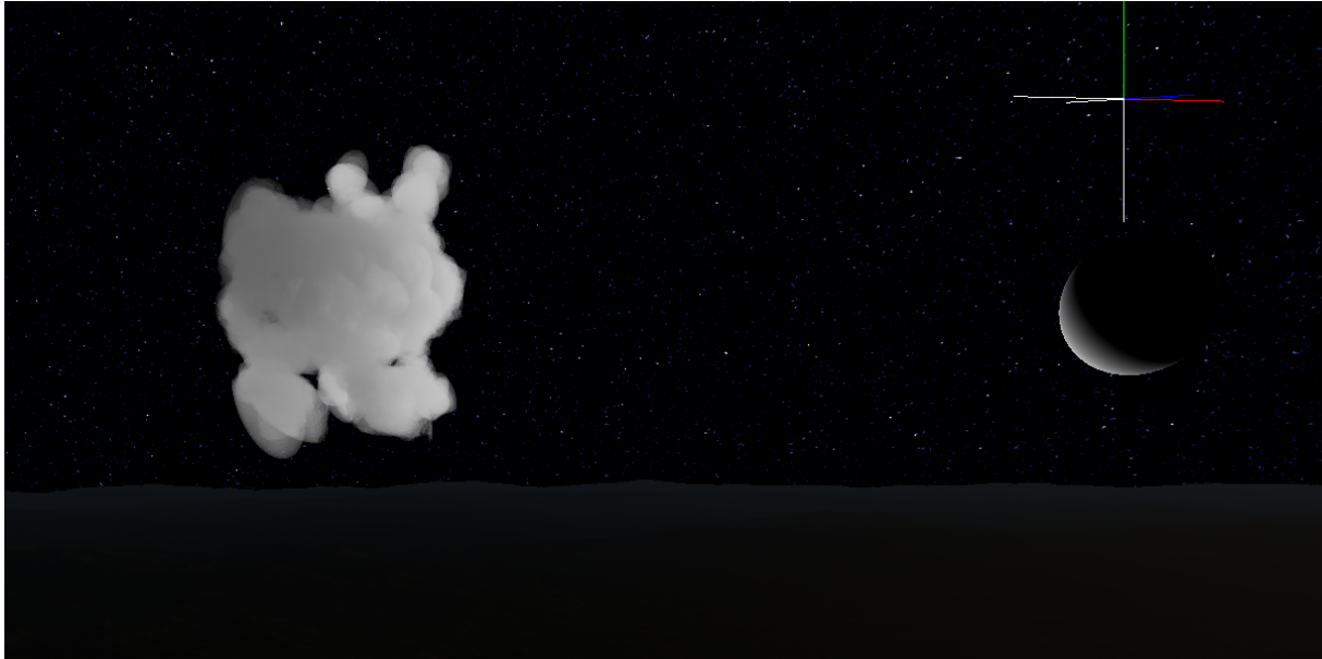
Figure 6.15. A rabbit mesh with 370 triangles. 80% decimation has been performed on this mesh, reducing the number of triangles from 1850 to 370 to achieve a suitable real-time performance.
