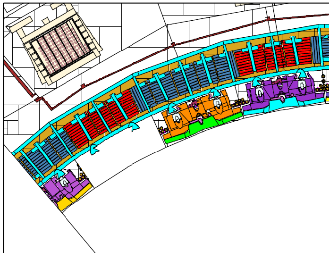
Figure 3-18. Missing blanket in row #13. The blanket universe was not allocated to any envelope cell in the NBI model.
