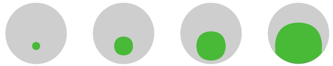
Fig. 3. Visualization of the utility introduction in the frontwave propagation for selecting the next goal. The gray circle represents a reachable area. The absence of obstacles allows the emerging frontwave to freely evolve from the robot position (slightly displaced downward relatively to the center of the circle) till the borders of the gray area, which in this particular case represents the boundary between explored and unexplored regions.
